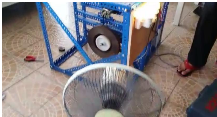
Figure 5. Functional Testing Of The Prototype With Connected Electrical Loads
