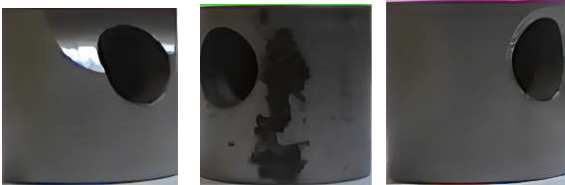
Figure 3. Piston dataset, (a) Defected 1, (b) Defected 2, (c) Normal
